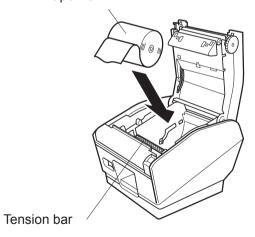
**Note:** Make sure not to pass the paper under the tension bar. In the following condition, remove the tension bar unit in accordance with the procedure described in paragraphs 3-7-1:
